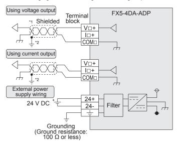
$V\Box +$ ,  $I\Box +$ ,  $COM\Box$ ,  $CH\Box$ :  $\Box$  represents the channel number.
