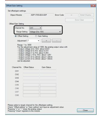
**2.** Select the target module for the offset/gain setting, and click [OK] button.
