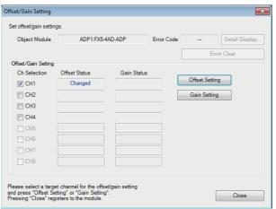
**2.** Select the target module for the offset/gain setting, and click [OK] button.
