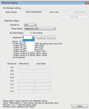
**5.** Use the radio button to specify whether to perform the offset setting or gain setting. (Step 6 and later describe the case when the offset setting is specified.)
