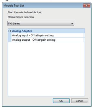
**1.** Select "Analog Adapter" ⇒ "Analog output - Offset/gain setting" and click the [OK] button.
