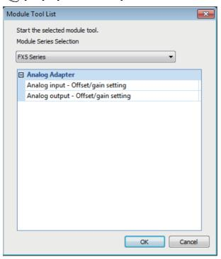
In "Analog Adapter", select "Analog input - Offset/gain setting" and click [OK] button.
