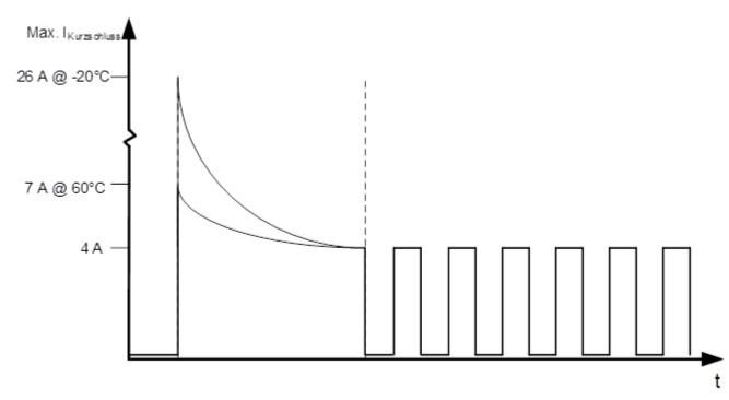
The unit limits the short-circuit current. The maximum short-circuit current depends on the ambient conditions and the operating state.
